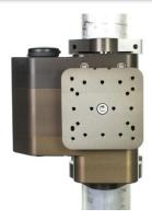
The QLA-60EBP-10 is a Power Over Ethernet (PoE) antenna positioner designed from the ground up to point and automatically peak directional side arm mount antennas for millimeter wave 70–90GHz (E-Band) links.
